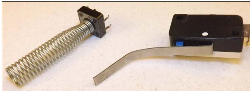
Small micro switches can be used as collision sensors
