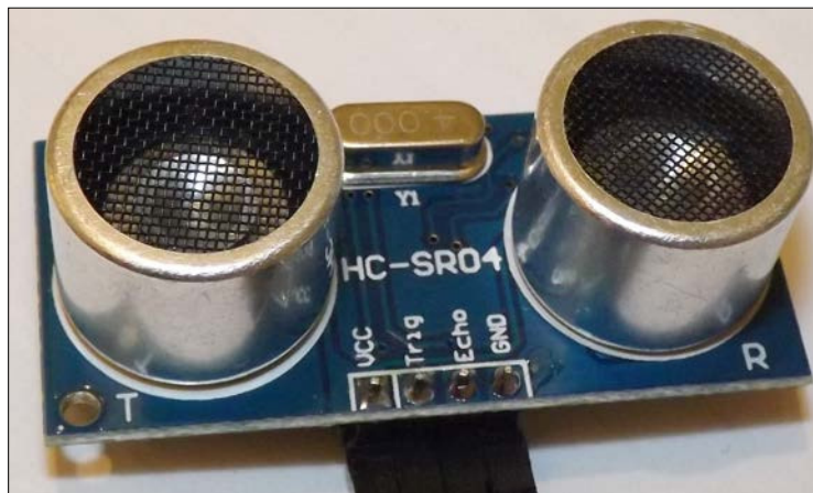
The HC-SR04 ultrasonic sensor module
