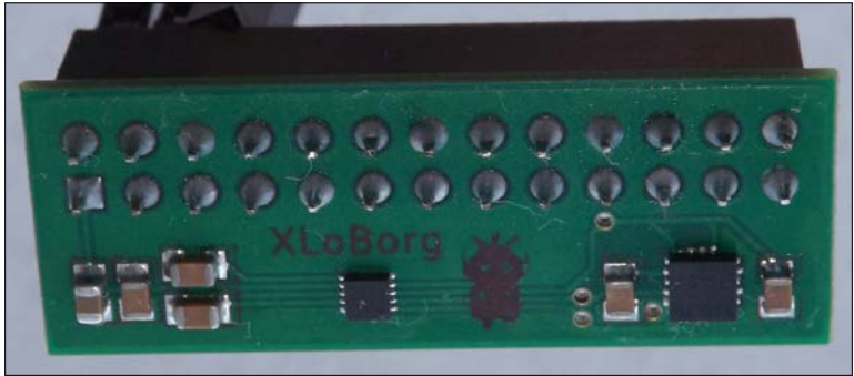
The PiBorg XLoBorg module contains a 3-axis magnetometer and accelerometer
